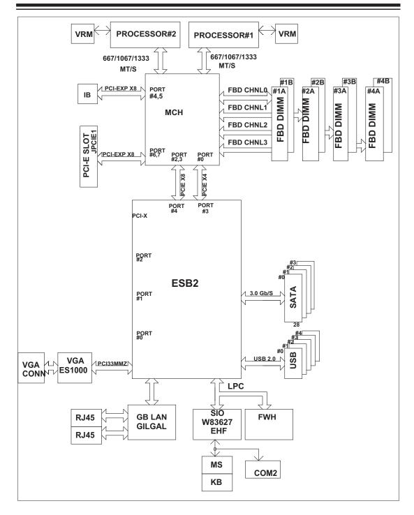
Figure 1-9. Block Diagram of the Motherboard
